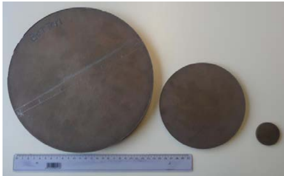
Fig. 1. 250 mm Diameter ZrO 2 -TiN blank shown next to smaller 150 mm and 40 mm blank.
