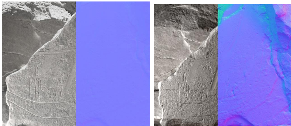
Fig. 7 – Comparison of the use of two different light sources to establish the most suitable approach in the field for the use of the Highlight RTI technique in open air. Both figures visualize the same Predynastic panel at el-Hosh (site: GYU-KING). To the right, a much brighter, but more heavy flashlight on battery was used. The left example demonstrates the result with a less bright, but lighter in weight, speedlight. The normal map shows how the speedlight produced insufficient power to detect all the characteristics of the rock relief, arguing for the usage of the flashlight on battery, © Belgian Archaeological Mission to ElKab.
