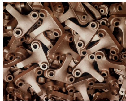
Figure 2. Objects supplied in bulk are stacked randomly in a bin. An object detection and pose estimation algorithm is needed to determine the six degree of freedom pose of a pickable object, so that it can be grasped by the robot.
