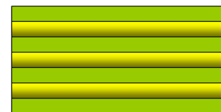
Figure 4: Inter-layer hybridisation schematic
