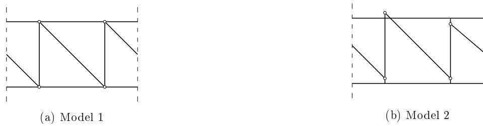
Figure 2: These figures show the two different analysis models. Model 1 is a statically determinate truss model where all members are pin connected. Model 2 is a statically indeterminate truss model where the chords are continuous and the braces are pin connected with infinitely stiff members.
