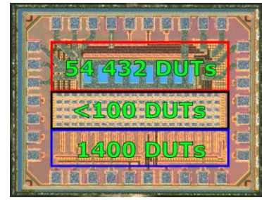
Fig. 4. Microphotograph of the chip with (top) the large array, (center) single FETs and (bottom) the pipelined array [6]-[7].
