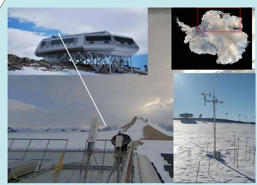
Figure 3: Remote sensing instruments and Automatic Weather station at Princess Elisabeth base
