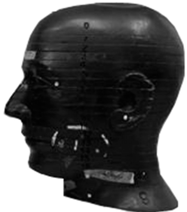
Figure 2 Anthropomorphic skull phantom (RANDO®; The Phantom Laboratory, Salem, NY), head and neck portion.
