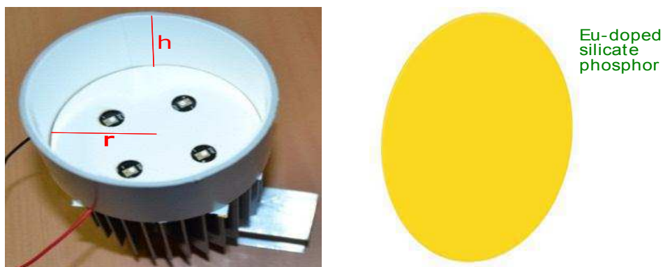
Fig. 1. Test sample of a remote phosphor LED module. Left: mixing cavity (radius=35.4 mm, height=43 mm); Right: remote phosphor converter plate
