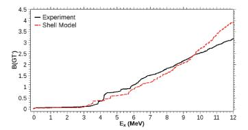
FIG. 6. (Color online) A comparison of the summed B(GT) strengths from the  ${}^{47}\text{Ti}({}^{3}\text{He},t){}^{47}\text{V}$  measurement (solid line) and the SM calculation using the GXPF1 interaction (dotted line) as a function of excitation energy.
