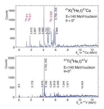
FIG. 8. (Color online) Comparison of (a) the  ${}^{41}\text{K}({}^{3}\text{He},t){}^{41}\text{Ca}$  spectrum and (b) the  ${}^{47}\text{Ti}({}^{3}\text{He},t){}^{47}\text{V}$  spectrum measured at 140 MeV/nucleon and 0°. The scales of the ordinates are adjusted so that the states with the same B(GT) value have the same height in these two spectra.
