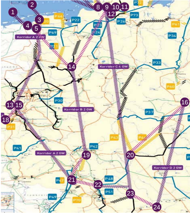
Figure 5: Development plans of the German TSOs [15] with some additional circuits (lighter purple with straight segments)
