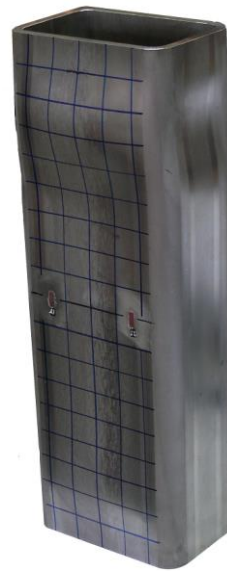
Fig. 7. Stub column failure mode of specimen RHS 150×100×6-3A.
