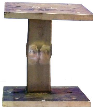
Fig. 15. Typical failure mode from biaxial bending plus compression tests (SHS 100×100×5-1I: e_{0y}=20\text{mm} , e_{0z}=60\text{mm} ).
