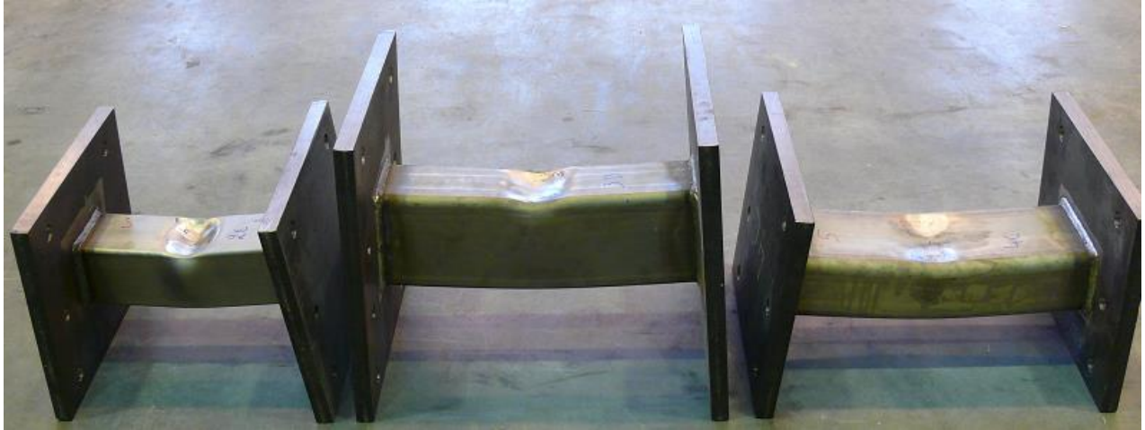
Fig. 14. Typical failure modes for uniaxial bending plus compression tests (from left to right: SHS 100×100×5-1D, RHS 150×100×6-3D, RHS 150×100×8-4D).
