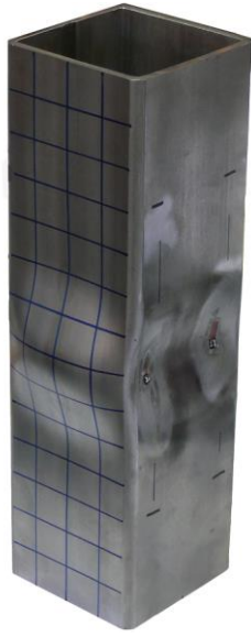
Fig. 6. Stub column failure mode of specimen SHS 100×100×5-1A.
