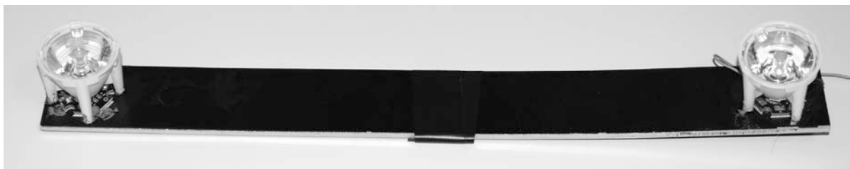
Figure 1 – The LEDs of the array used in the experiments, are rotated by bending the aluminum support. The distance between the centers of the LEDs ( D_{Array} ) is 0.32m.
