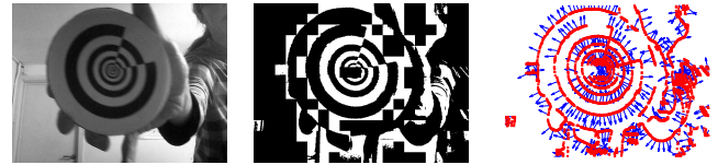
(a) Image from a scene with the marker. (b) Black-and-white image after local thresholding of 4(a). (c) Edges and gradients extracted from respectively 4(b) and 4(a). Only 10% of the gradients is shown.
