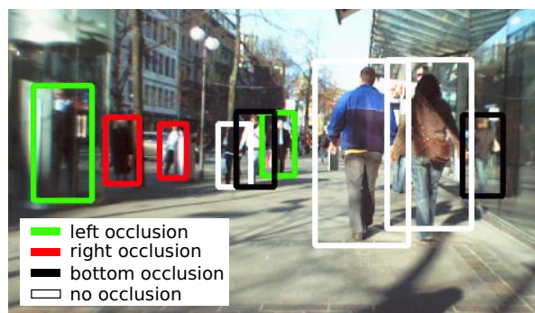
Figure 1: Motivation: to handle frequently occurring occlusions, we train many occlusion specific classifiers.
