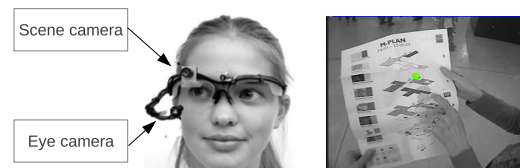
Figure 1: Left: illustration of a mobile eye-tracker consisting of a scene camera and an eye camera. Right: output of a mobile eye-tracker in which the data of the scene camera and the captured gaze point (green dot) are combined.
