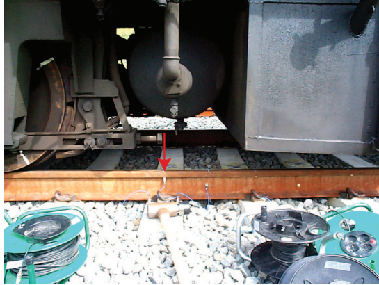
Figure 3.27: View of the measurement setup for the determination of the track receptance in loaded conditions. The impact location F1 is indicated by the red arrow.
