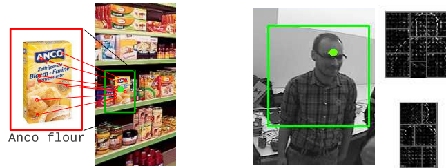
Fig. 2 Illustration of our matching techniques. Left part of the image illustrates the object correspondences. Right part illustrates a person detection and our model for torso and upperbody detection.
