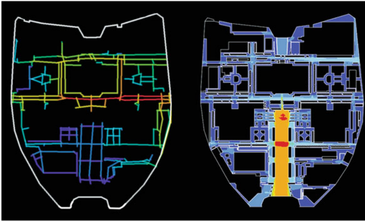
Fig. 2 (From left to right) axial map of IST campus, excluding stairs. Integration—min: 0.26 (dark blue); max: 0.68 (red). VGA connectivity—campus with car parking as barriers—min: 1 (dark blue); max: 5571 (red); grid: 3 m
