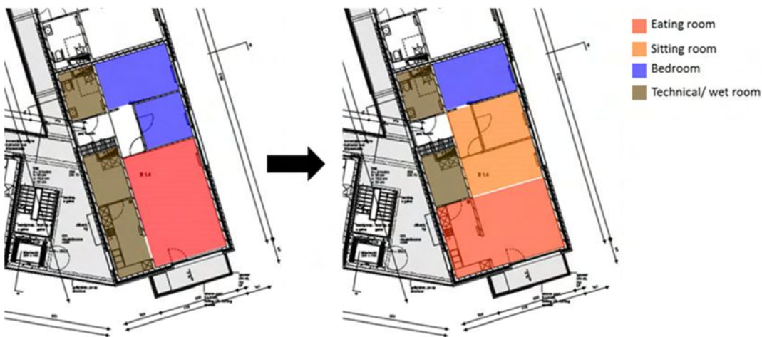
Fig. 12: Renovation scenario 2 (transformation from two-bedroom apartment to one-bedroom apartment) [2]
