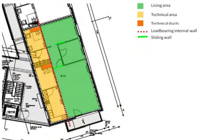
Fig. 7: Flexibility of the analysed housing unit [2]
