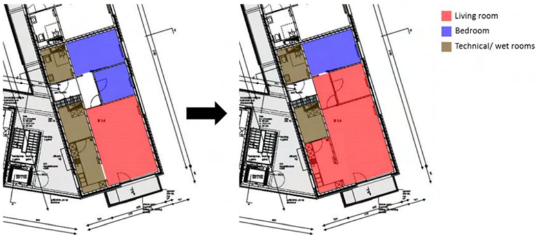
Fig. 8: Renovation scenario 1 (transformation from two-bedroom apartment to one-bedroom apartment) [2]
