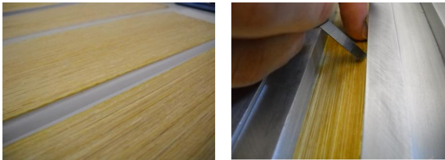
Figure 1. a) Bamboo UD preforms ready to be used and b) positioning the preforms in the mould.
