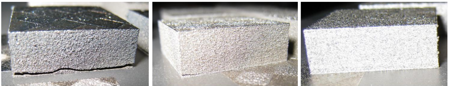
Figure 5: M2 HSS parts produced with a pre-heating temperature of 90°C (left), 150 °C (middle), 200 °C (right)
