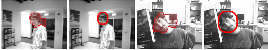
Fig. 6. In contrast to the image segmentation based tracker using hough transform (HTT, 1 st and 3 rd column) our approach (2 nd and 4 th column) based on Dynamic Objectness includes motion information which is often a more dominant cue.
