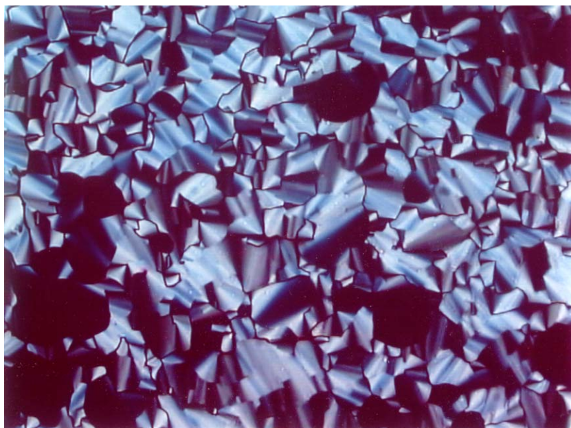
Figure 3: Texture of (C_{16}H_{33}O)_8PcCo between crossed polarizers in the hexagonal columnar mesophase.
