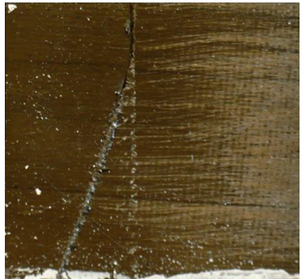
Fig. 10. Failure of off-axis [15]_{10} under compression loads.
