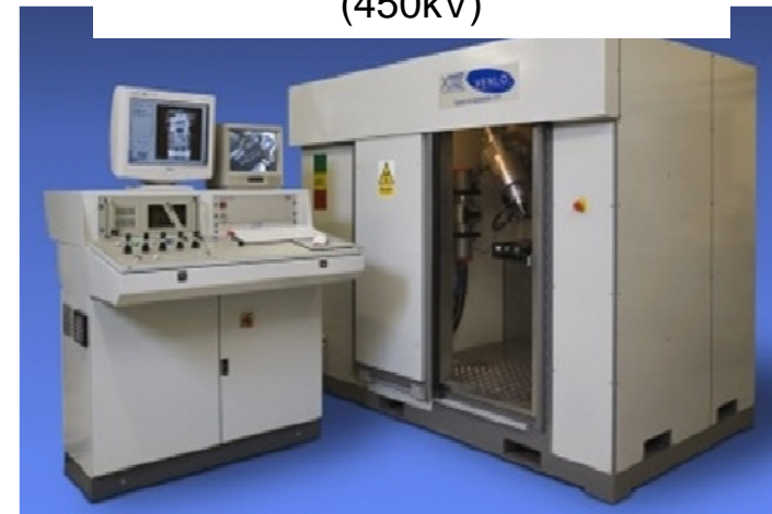
X-ray CT tomograph for dimensional measurement (450kV)
