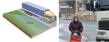
Figure 1. Blind spot area of a truck
