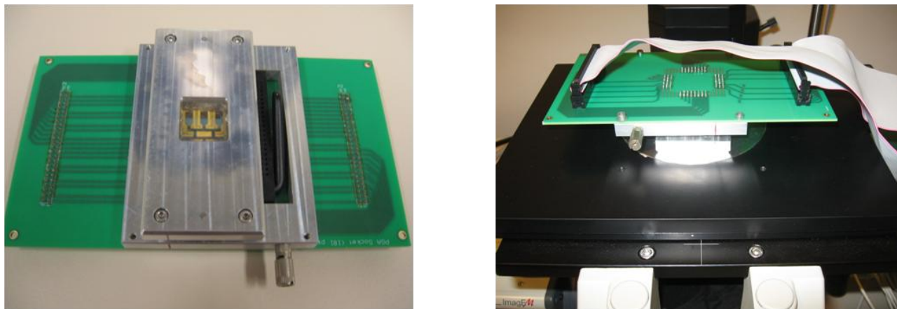
Figure 1: Image of the digital lab-on-a-chip placed in the specially designed chip holder (left) suitable for use on the inverted fluorescence microscope (right).
