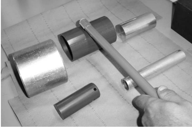
Figure 4.7: Experimental setup to evaluate the integrated system. The experimenter manually rolls the tactile sensor over cylinders of different size. The test subject is positioned at the opposite side of a screen and has to say which cylinder is bigger.
