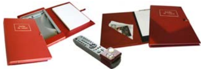
Figure 2 The Piece of Family working prototype: a notebook with a scanner in its cover, and a small extension to the television's remote control.
