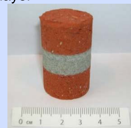
Test sample – d=29mm – h=48 mm
