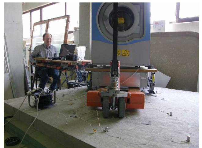
Fig.2 Washing machine mounted on heavy concrete base on steel feet on the RP. Also visible are the jacks (supporting the MDF plate) and the rubber replacement feet (on the MDF plate).
