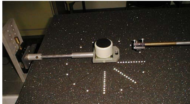
Figure 5. Typical setup for the measurement of the elastic moduli using surface waves.
