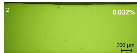
35 A, 200 mm/s, a_1=0.1 , three re-melting scans
