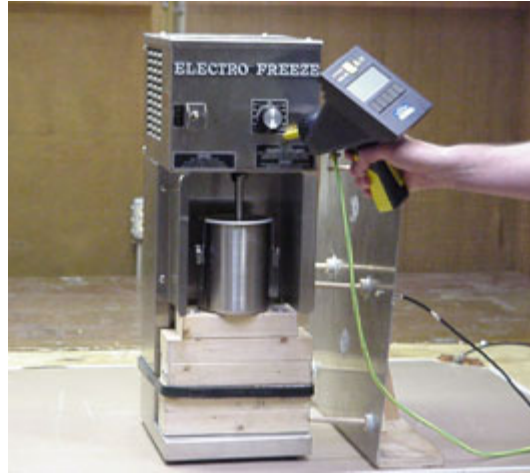
Figure 2.9: IEC 61000-4-2 testing being performed. [Courtesy of DLSEMC]
