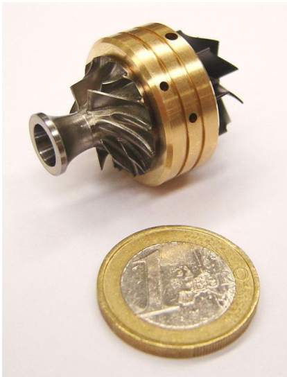
Fig. 3. Compressor (left), turbine (right) and air bearing insert. Rotor diameter: 20 mm. Size compared to 1 euro coin.
