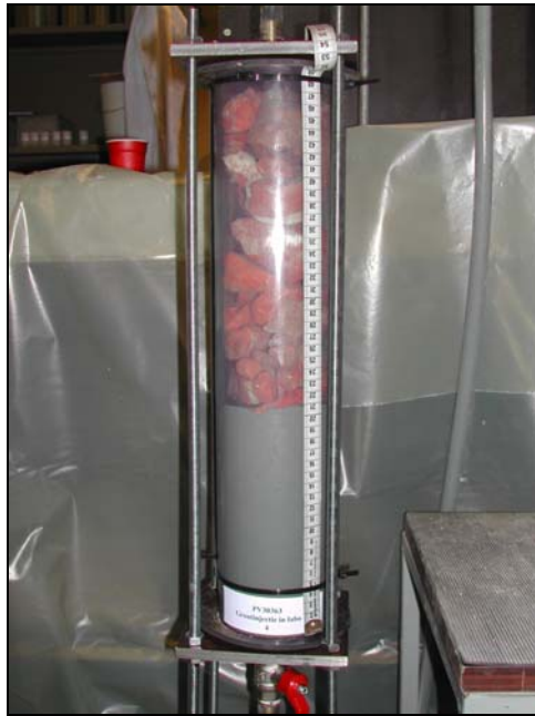
Fig.5 -- Injection with grout (composition 3) under a hydraulic fall of 1 m of a tube, filled with brick material from the site. The curing period was 28 days.
