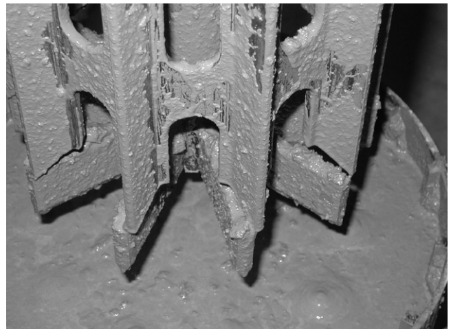
Fig. 2. Detailed view of inner cylinder upper and bottom unit of the ConTec Visco5 (here: immediately after testing a SCC mixture).
